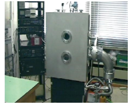
High vacuum pumping system and vacuum chambers for the preparation of thin films with thermal evaporation and electron beam deposition.
